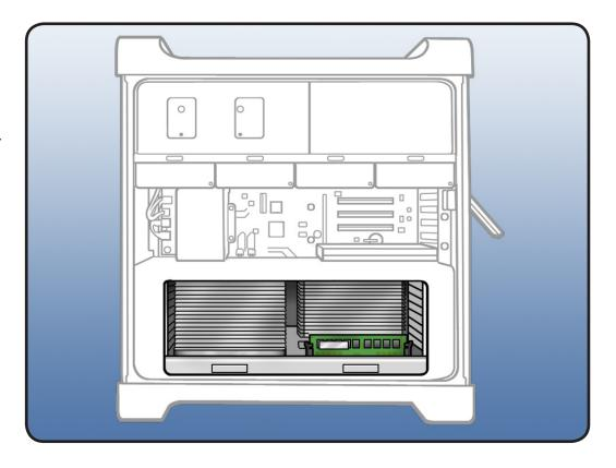
Press down and release 2 latches on front of processor tray.
